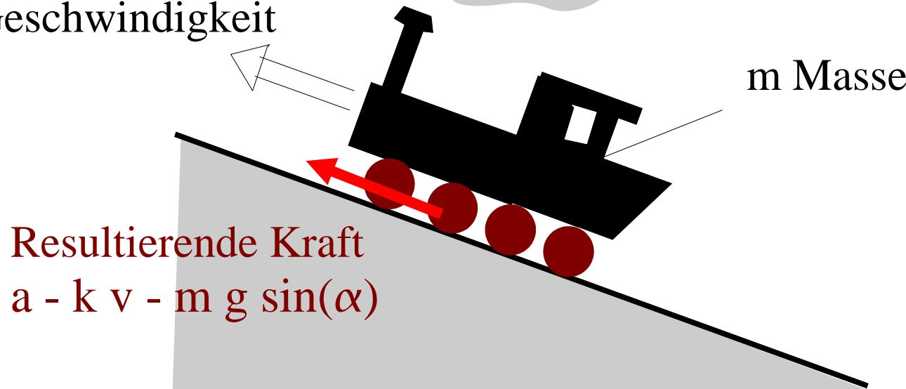
$$\begin{aligned} \text{Masse} \times \text{Beschleunigung} &= \text{Kraft} \\ \mathbf{m} \mathbf{v}'(\mathbf{t}) &= \mathbf{a} - \mathbf{k} \mathbf{v}(\mathbf{t}) - \mathbf{m} \mathbf{g} \sin(\alpha) \end{aligned}$$
