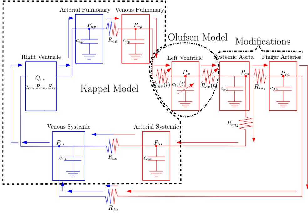
FIGURE 2. The cardiovascular model showing the (Kappel) non-pulsatile global model, (Olufsen) pulsatile left heart model and the model modifications.
