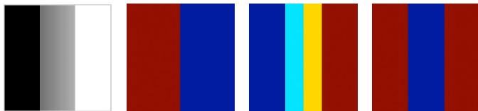
Figure: Comparison between the standard recursive bi-partitioning method and our method: (a) Original image. (b) segmentation after 1st bi-partitioning. (c) segmentation after 2nd/final bi-partitioning (over-segmentation). (d) Our algorithm (correct segmentation).
