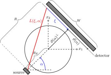
Geometry for the fanbeam transform. The line  $L(\alpha, \xi)$  connects the source and the detector, both rotated by the angle  $\alpha$ , at detector offset  $\xi$ . The values R and  $R_E$  denote the distances from the emitter to the detector and origin, respectively, while W denotes the detector width.
