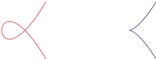
Figure B.2: The node with equation x^2 = y^2 + x^3 and the cusp x^3 = y^2 .
