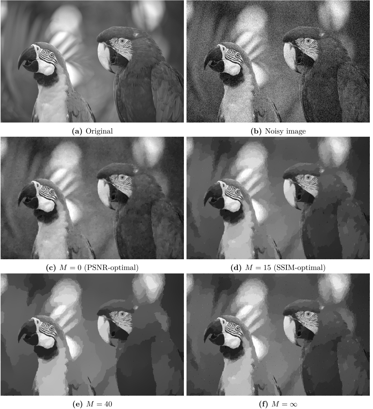
Figure 5: Parrot photo: denoising results with noise level \sigma = 30 (Gaussian), for varying cut-off M , fixed q = 0.5 and fixed \alpha^\infty = 0.0253 .
