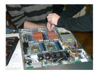
We pulled the plug again and reopened the case to check again if all parts were correctly installed and connected. We first suspected some wrong jumper configuration to be the problem, but could not find any errors. So we tried to switch it on again but first removed three of the processors. Now, with only one processor, the PC worked perfectly fine.
