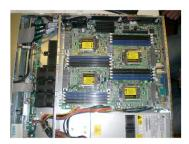
With all parts (hopefully) correctly installed, we closed the case and attached monitor, keyboard, mouse, and the power cord. Then we finally switched the computer on the first time. Sadly, apart from the fans starting to run and some blinking LEDs nothing happened (no output signal on the screen).
